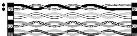
The wiring fault **reversal** indicates that the pins of **one** twisted pair is connected incorrectly.
