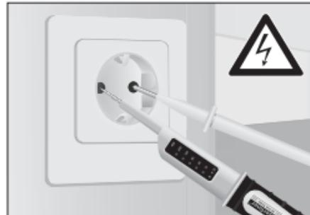
If voltage is present, all the LEDs up to the voltage measured will light up, along with the positive and negative LEDs.
