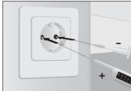
Hold the base device (+) in your right hand and the second test prod (-) in your left hand. Now apply the test prods to the contacts to be tested (line, socket, etc.).
