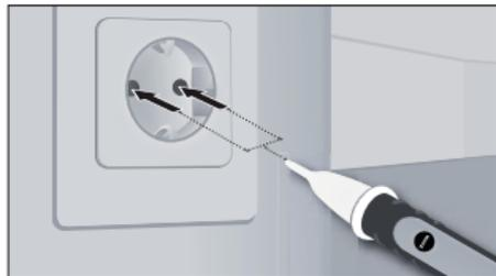
Position the detector tip in the area to be tested (e.g. cable, socket. etc.).
